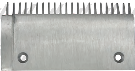
PF120011 (ALUMINUM) LH - 22T - 203mm - 2 RAISED TEETH - 2 HOLE GS8000 ESCALATOR
