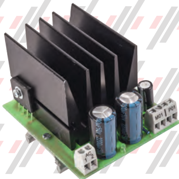
PSSSG897220 POWER SUPPLY BOARD 9300 ESCALATOR
